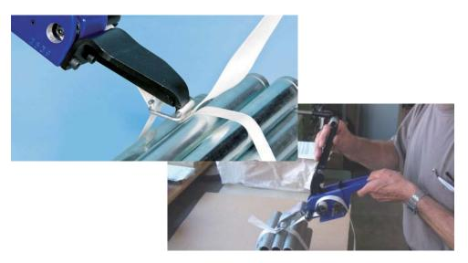
The specifically for the ManuCord MRC developed accessory provides a simple way for fast and reliable strapping of all packages, that have no alternatively only small contact face.
