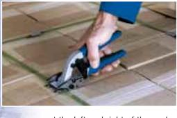
at the left and right of the seal, cut the strap, and hold the seal between the two blades. This saves time and money!
